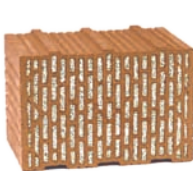
Mineralfaserdämmung, lose \lambda = 0,10 \text{ W/mK} R_{w,1} = 52,2 \text{ dB} f_k = 5,0 \text{ MN/m}^2 (bei SFK 12)
